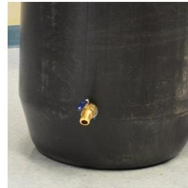
Next, crawl inside your barrel to seal the faucet. Press rubber gasket tightly against faucet/barrel wall, follow with big washer (indented side towards barrel) and screw on lock nut. Tighten lock nut with pliers. Using a flashlight is helpful. The faucet is now connected.
