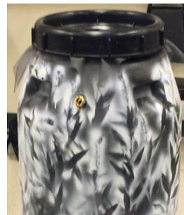
Screw in the adapter using a wrench, making sure to protect the threads and place in lock nut. Use pliers to tighten, making sure to cover threads with a rag or pipe cap to prevent damage.
